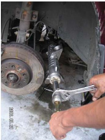
PIC 5: Removing the inner rod
