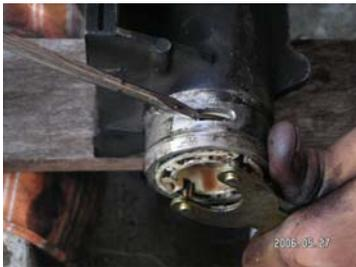
PIC 9: Removing the locking pin
