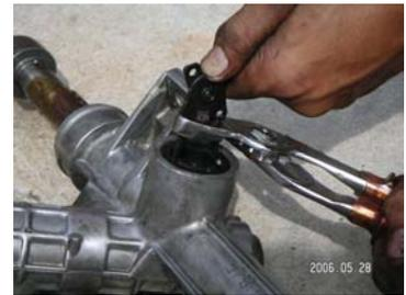
PIC 10: Removing the rear plug
