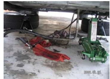
PIC 1: Support the car with 2 jack stand, with hydraulic jack supporting the transmission body
